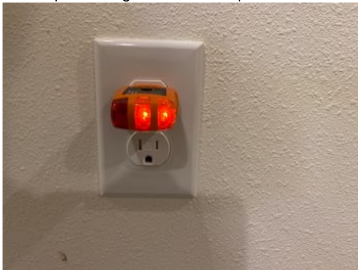
Example of un-grounded GFCI protected outlet
